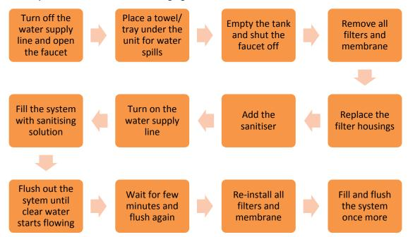
Fig. 5.3.8: Steps to sanitise an RO system
