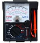
It consists of a needle which points at the scale built on it for giving the measured value.
