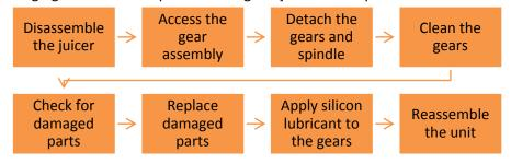
Fig. 6.2.6: Servicing the juicer drive system
