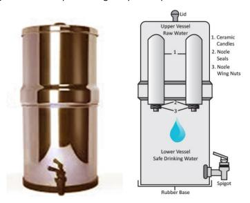
Fig. 5.1.21: Gravity based purifier
