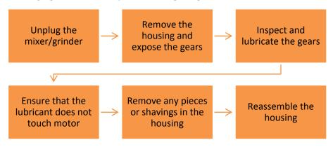
Fig. 6.2.2: Servicing the gears
