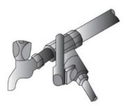
Fig. 5.2.6: 3-way connector connected to the water supply
